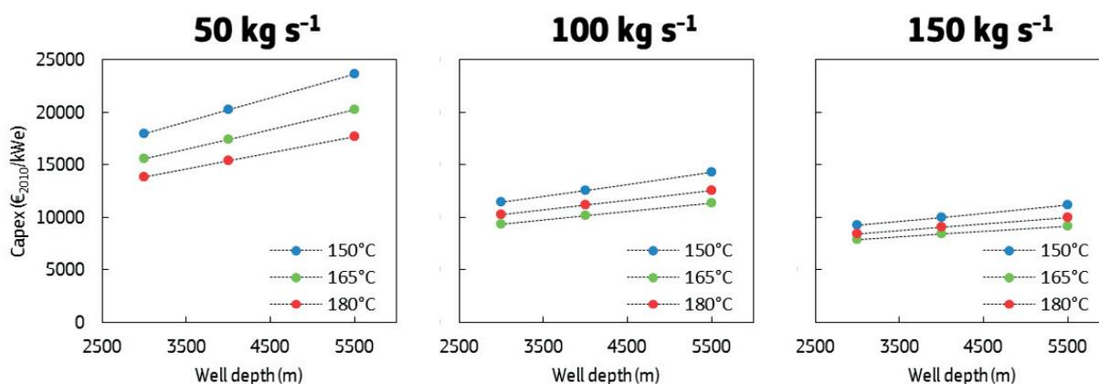
Fig. 39: Influence of well depth and pump rate on CAPEX of an ORC EGS power plant. It may be much more cost effective to increase the permeability of a reservoir between injection and production wells than to drill deeper for higher reservoir temperatures. Source: JRC own analysis with GeoELEC software [Dauenhauer 2014]
