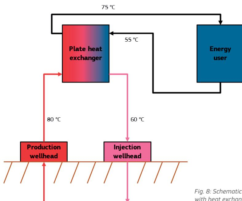
Fig. 8: Schematic process flow diagram for a direct use system with heat exchanger. Source: [Lund 1998], adapted
