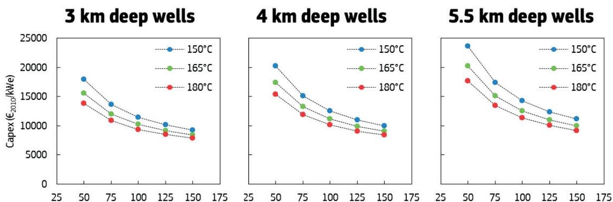
Fig. 38: Influence of pump rate (and therefore permeability) on the CAPEX of an EGS ORC power plant. The reference case provided is that of 5.5 km deep wells, 100 kg/s pump rate and 165°C inlet water. CAPEX numbers are those generated by the model and have not been corrected for the CAPEX brake down used. Source: JRC own analysis with GeoELEC software [Dauenhauer 2014].
