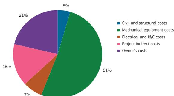
Fig. 36: CAPEX breakdown of a hydrothermal flash power plant
