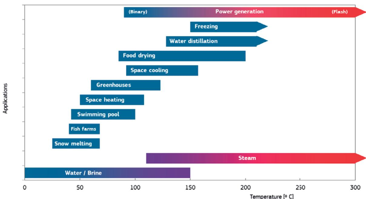
Fig. 3: A Lindal diagram of temperature of geothermal water and steam suitable for various applications
